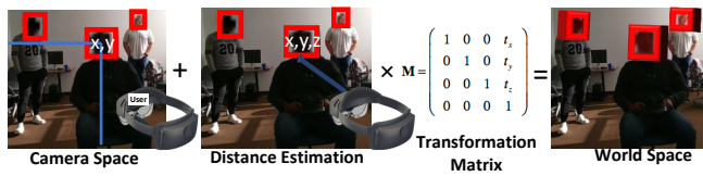
Figure 3: An illustration of the 2D-to-3D camera-to-world transformation process. Here, matrix M is an arbitrary transformation matrix created from the metadata included with each captured frame; it is used to convert 3D points in camera space to world space.
